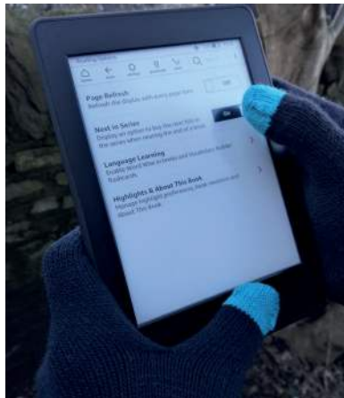
Figure 2: Swipegloves can be used with touchscreens
